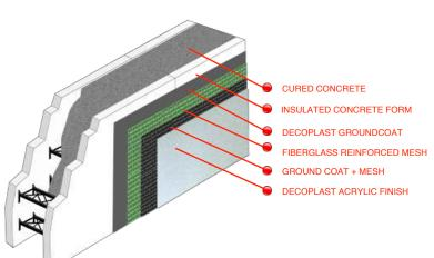
The Deco Direct Insulated Concrete Form System (DDICF) is a unique, energy efficient system thats has been engineered to be directly applied over insulated concrete forms. These lightweight forms are set into place at the job site and braced together. On its own, they are too light to bear any weight, however once filled with concrete and after they have cured, they are ready to be finished.
