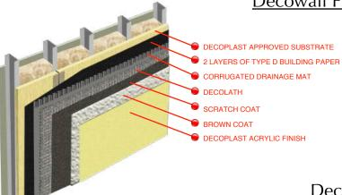
The **Decoplast FRS Drainage System** is a heavy-duty solid transitional stucco system that drains incidental moisture to protect any structure from harsh elements.
