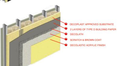
The Decoplast Decowall FRS System is a traditional cement stucco system that consists of lathing, scratch coat, brown coat, and a Textured Finish Coat.
